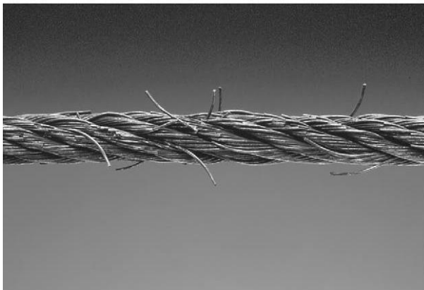
Cable With Severe Corrosion
