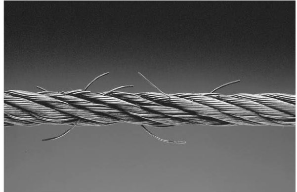
Cable With Broken Wires
